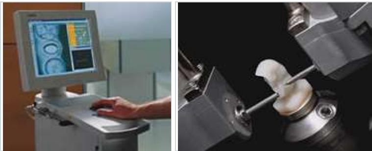
*CEREC computerised design unit (left), and milling unit (right).*
